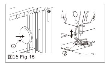
Press needle gauge knob ① and rorate it a -ccording to arrows, do not release it until the the number you require aim at A direction right above machine head, Loose needle gauge kn -ob ①.
